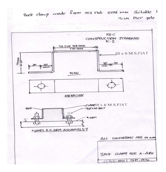
11KV V Cross arm (75x40) with clamp for 9.1Mtrs PSCC Poles
