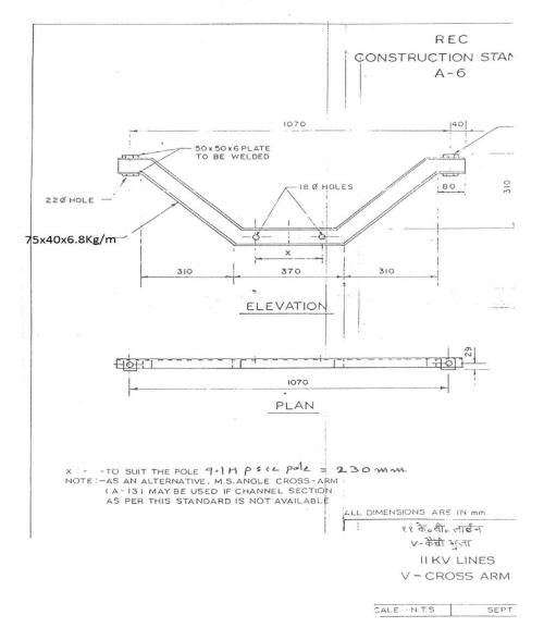
11KV V Cross arm (75x40) with clamp for 9.1Mtrs PSCC Poles
